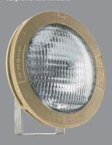
UWF 22 high power 300W PAR 56 extra low voltage (12V) underwater floodlights. Suitable for permanent submersible installation into depths between 0.3 - 5.0 metres. UWF 22 fittings are especially suited for swimming pools, water displays and fountains, creating dramatic and exciting effects.
