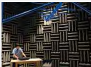
Acoustic radio wave anechoic chamber
