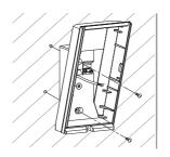
4 Install main unit after wiring to the terminal.
